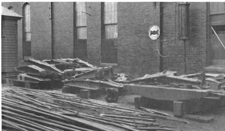
Adjoining the new oxy-acetylene plant at Kansas City, Mo. On the left, finished bolsters; at right, bolsters unfinished. Center shows air hoist from gib crane. Underneath is narrow gauge track and car which runs into the shop and serves three operators.
